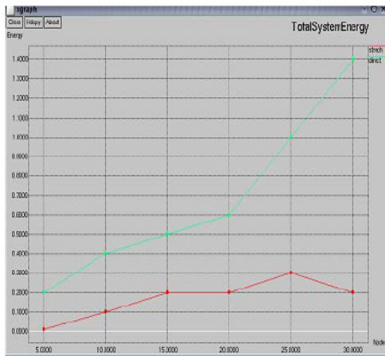
Fig.4 Total system energy for always-direct system and stretched system with BS at center
